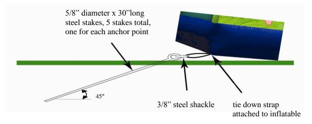
If the unit is on cement or any hard surface, to protect the base or the unit from abrasion, make sure that you have put a tarp down and placed the unit on it before inflating it. Use sand bag pouches that can carry a minimum of 200 lbs tension load per anchor point. Connect the tie down straps to the sand bag pouches. Remember to install sand bags at such distance from the ride that the ride straps connected to the shackle would be taut.
